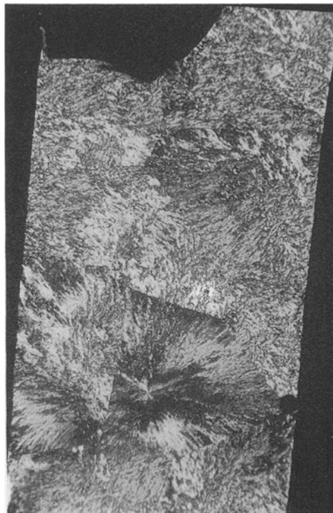
Plate 1: Polarized Optical Microphotograph of a Thin (0.7 mm) Section of a POM DSC Sample, after Crystallization at 157.0 °C
